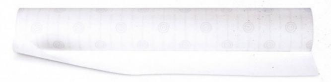
ThinFire is a ceramic-impregnated shelf paper that provides excellent separation between glass and kiln shelf in firing applications up to 1600°F (871°C). Compared to more conventional ceramic fiber materials, it produces a glossier finish on the shelf side of your project, creates less binderburnout odor, and is lighter in weight (for easier handling and storage). Compared to kiln washes, ThinFire reduces shelf preparation time and improves surface release.
